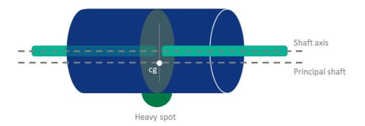
Rotor balancing is a vital aspect of the maintenance routine for a steam turbine (or its generator). Low-speed balancing is often performed on-site or in a facility that lacks access to a high-speed balance cell. Relying on the results of low-speed balancing can mean that maintenance engineers miss issues that surface only when the machine is run under full-speed conditions. Therefore, as the rotor must be in dynamic balance, at-speed balancing is the most effective way of achieving this.
