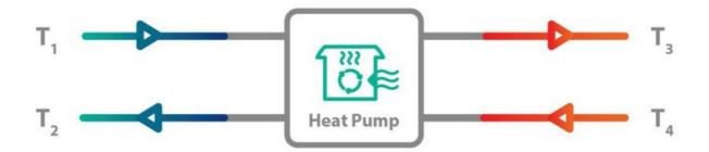
The heat pump system performance depends on the four temperatures shown in Figure 1 above: the flow and return temperature on the heat source  $(T_1, T_2)$ , and the flow and return temperature on the heat distribution system  $(T_3, T_4)$ . If these temperatures stay within the range required, the heat pump is likely to achieve a seasonal performance factor (SPF), be reliable and require very little maintenance.
