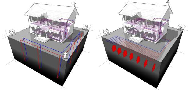
Figure 13: Typical configurations of ground-source heat pumps
