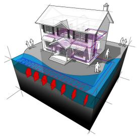
Both systems require an accessible body of water within a reasonable distance from the heat demand. You should assess the volume of the source, and whether it can provide sufficient heat over a year.
