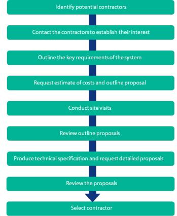
Figure 4.1: Process for procuring contractor
