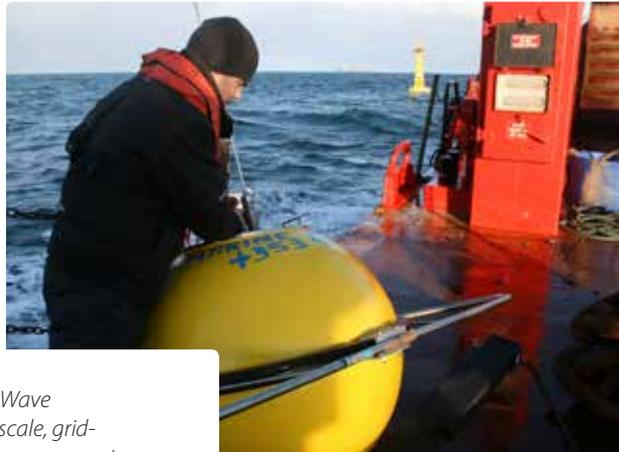
SEAI is giving €2.3 million grant aid to New Wave Technologies Ltd to design and build a full-scale, grid-connected version of their OE Buoy wave energy converter. The OE Buoy is a floating, oscillating water column-type wave energy device, incorporating a bi-directional air turbine, and is the first Irish-designed wave energy device to reach full scale. The prototype, with a rated capacity of 500 kW, will be 37m long, 17m wide, with a draught of 9.5m, weighing approximately 625 tonnes.
